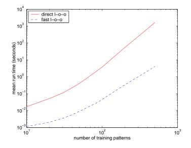
Figure 1: Graph of run-time as a function of the number of training patterns for leave-one-out cross-validation of kernel Fisher discriminant classifiers via direct and fast approximate methods (mean of 20 trials).
