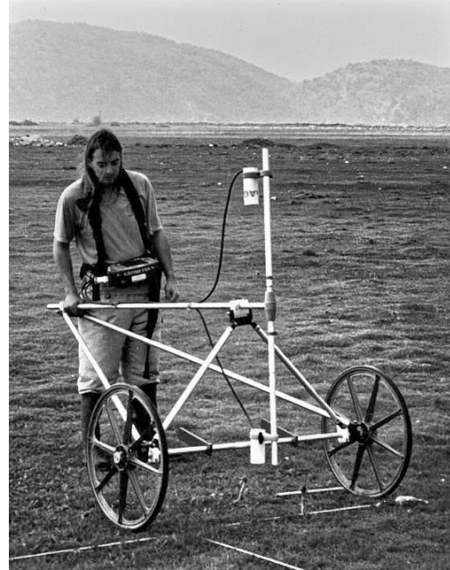
Fig. 1. One of the authors (DJB) performing the geomagnetic survey of the Roman suburb at the Butrint site in Southern Albania. Measurements were made at 0.25m intervals along lines 1m apart.
