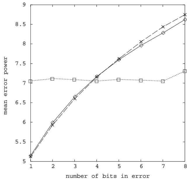
Figure 1: Graph of mean error power against Hamming distance, for an un-ordered codebook, and codebooks ordered using simulated annealing and quadratic assignment algorithms.
