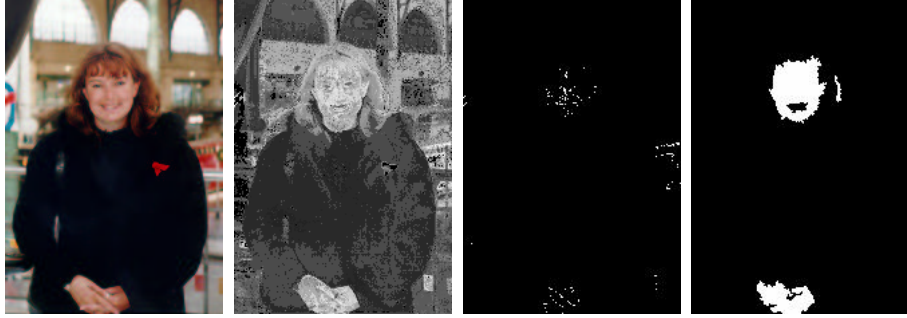
Fig. 1. Original image (left) and associated log-likelihood image (second from left) displayed so that the lowest non-zero likelihood ( \log L = -7.84 ) is black and the maximum likelihood, ( \log L = 4.99 ) is white; seed points for region growing algorithm (third from left) and final mask (right).
